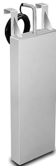
Tấm rung siêu âm hình bát giác, cực rung gần 2 mặt Octagonal ultrasonic transducer plate with transducer blocks mounted on two faces • Frequency: Customizable 28/40Khz • Power: Customizable 300W - 2400W • Size: Customizable according to tank design
