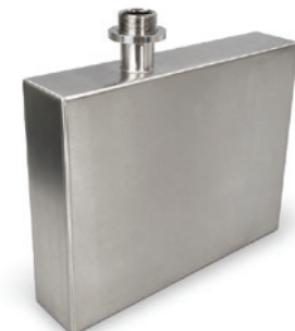
Tấm rung siêu âm nối với thành bể bằng mặt bích Ultrasonic transducer plate connected to the tank wall by a flange • Frequency: Customizable 28/40Khz • Power: Customizable 300W - 2400W • Size: Customizable according to tank design
