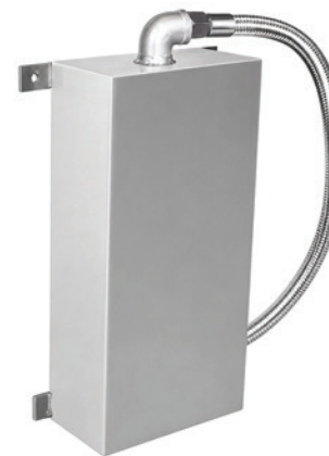
Tấm rung siêu âm nhúng - Kết nối ống mềm inox Immersible ultrasonic transducer plate – connected via a stainless-steel flexible conduit • Frequency: Customizable 28/40Khz • Power: Customizable 2400W • Size: Customizable according to tank design
